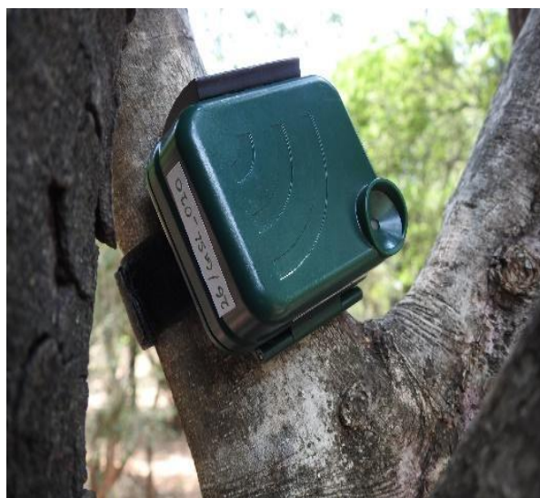
Figure 3. AudioMoth audio recorder labelled and deployed
